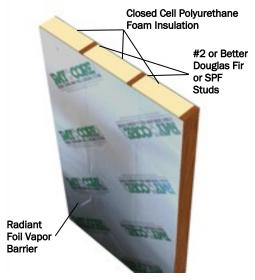
WALL OR ROOF PANEL - 3-1/2\*THICK PANEL, STUDS 16\* OC - R26
