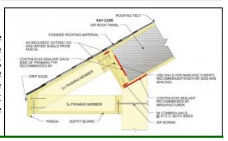
"Hot" Roof (Unvented) Application: Most shingle manufacturers today warrant their products for unvented roof application when properly installed, but it is recommended that you check with your shingle manufacturer to assure that this is an approved application. For unvented applications, simply apply roof deck materials, such as plywood or OSB, directly on top of the properly
