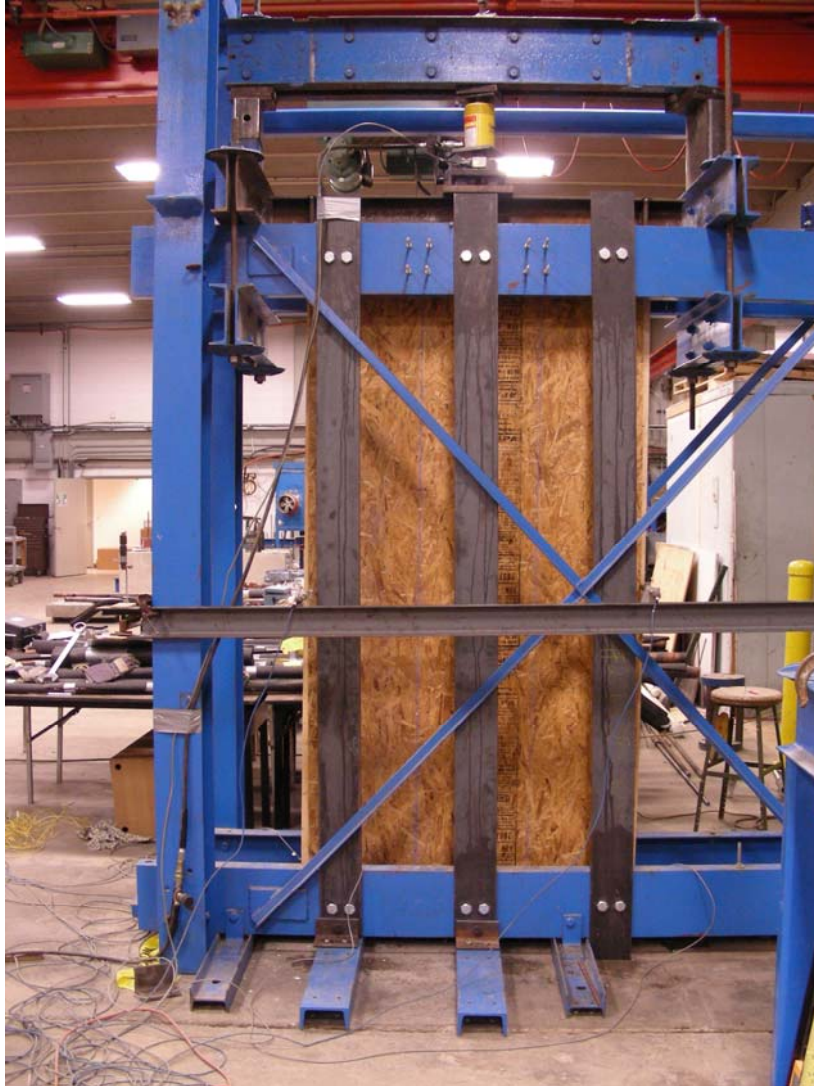
Figure 1. Side view of compressive load test set-up.
