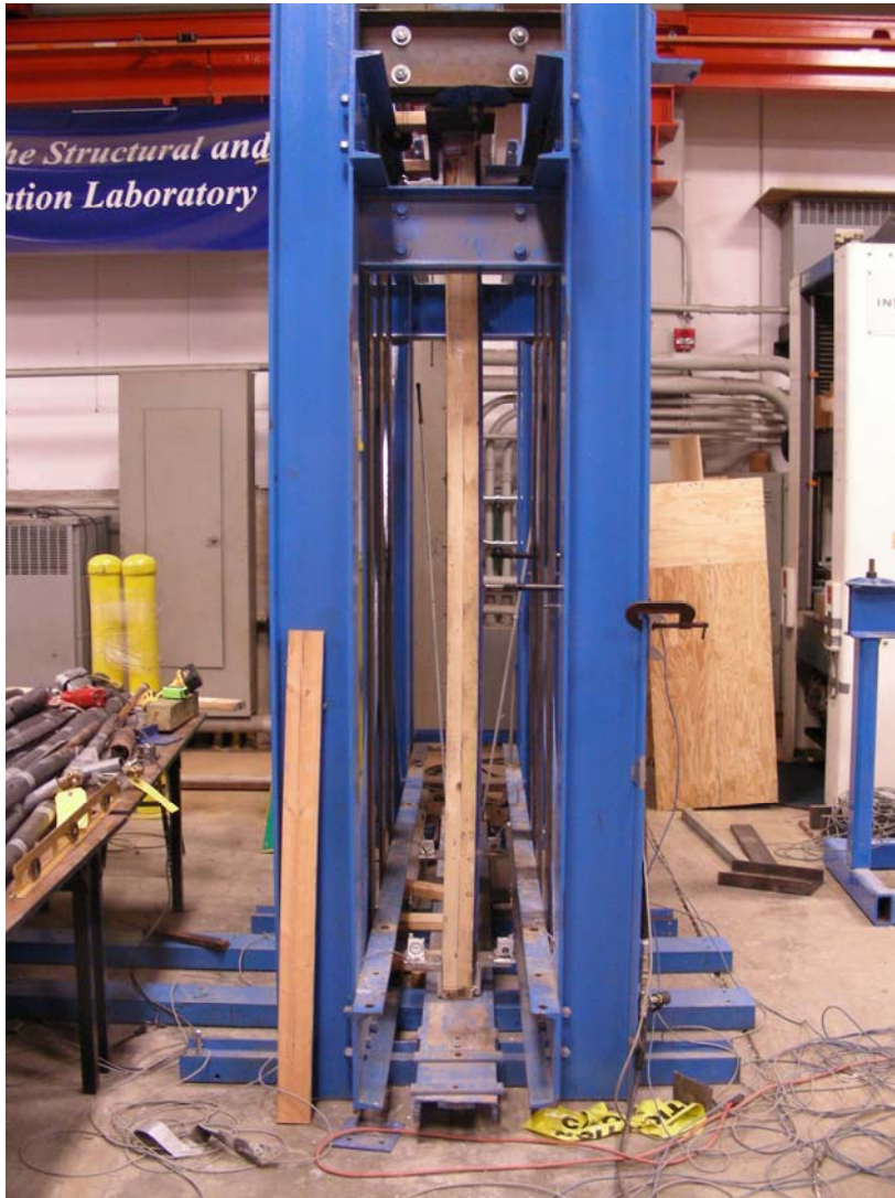
Figure 2. Front view of compressive load test set-up.
