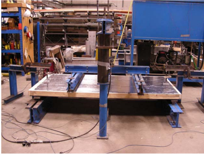
Figure 3. Transverse load test set-up.
